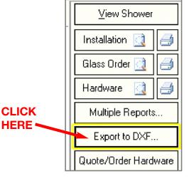
1) Showers Online now exports DXF files for automated cutting machines. Simply press the Export to DXF button on the shower list screen and save these valuable files. Once the files are saved, export them to the Computer Numerically Controlled (CNC) machine for the glass to be cut, polished, notched and drilled. This feature is a tremendous time-saver for companies who cut their glass using CNC machines.
